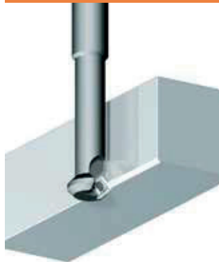
Rear surface Edge chamfering process
